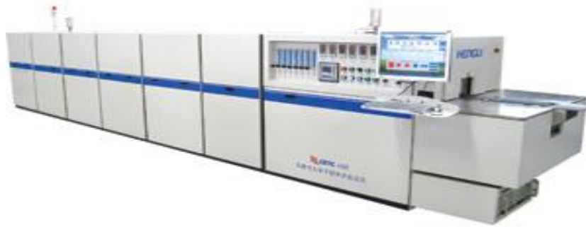
Figure 4. Hengli HSA series belt furnace
